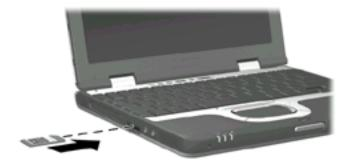
Inserting an SD card into the SD slot
